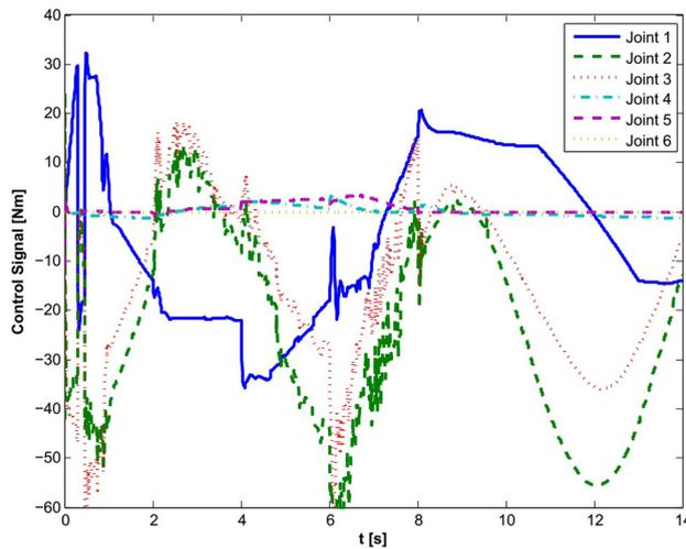
Fig. 15. Torque control signal for the proposed fuzzy gain dynamic surface (Case 1.2).
