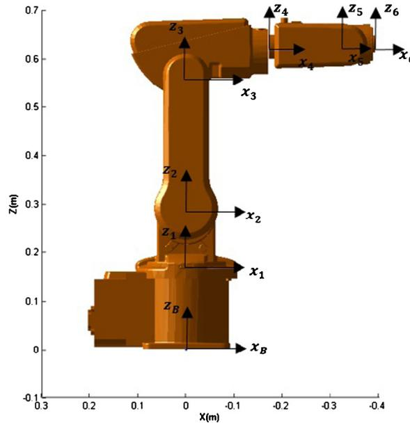
Fig. 6. Coordinate systems of ABB IRB 120 robot manipulator.
