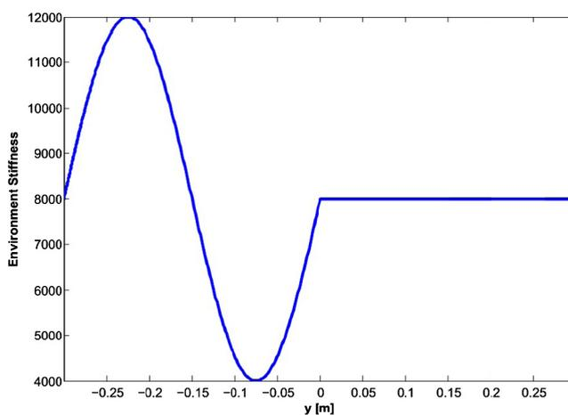
Fig. 8. Stiffness profiles for environments 1, 2 and free motion.
