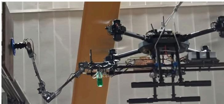
**Figure 1:** Indoor NDT inspection executed by an autonomous tilting aerial manipulator [7].
