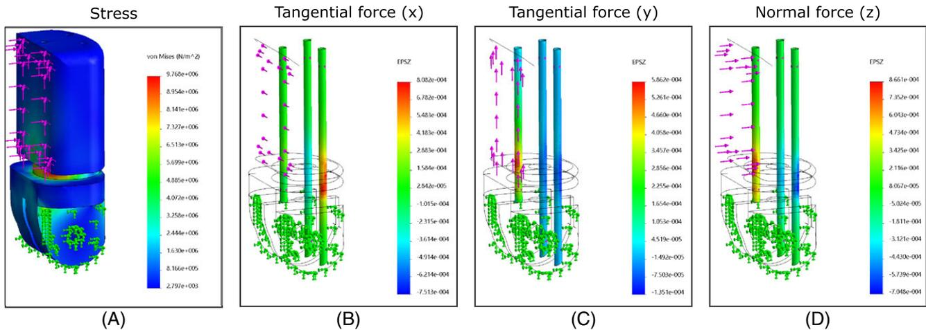
**FIGURE 8** Finite element analysis of the proposed finger sensor design. A, structure stress, (B, C, D) simulated deformation of the three Bragg fibers when the phalanx is subject to a normal, tangential and vertical force
