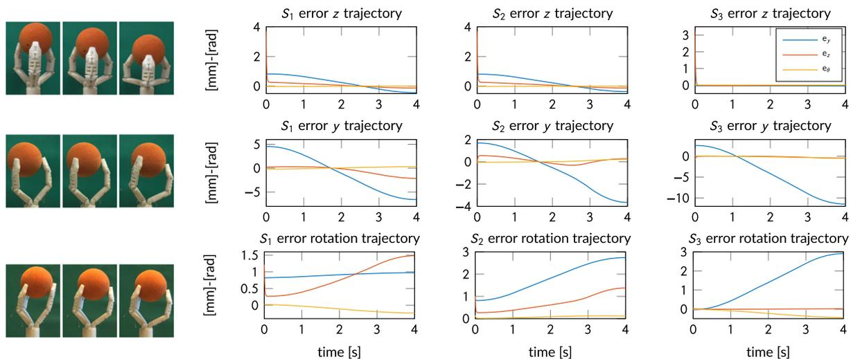
**FIGURE 2** Object errors in the Cartesian space for  $S_1$ ,  $S_2$ , and  $S_3$  for three different trajectories: along  $z$  direction, along  $y$  direction, and for the rotation in the  $yz$  plane. The left pictures are taken from real experiments performed on the prototype implementing  $S_1$  coupling matrix
