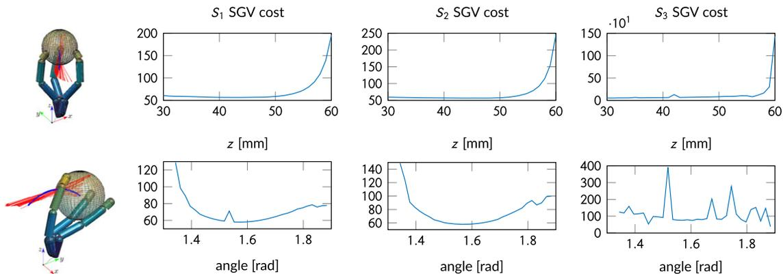
**FIGURE 1** SGV cost variations: along  $z$  direction (top) and along the circular path on  $yz$  plane with respect to the rotation angle (bottom). The red lines on the left are the principal directions of motion
