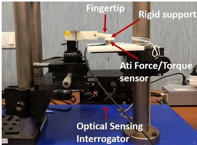
FIGURE 9 Measurement system
