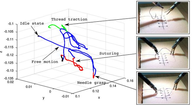
**Fig. 2:** Example of trajectory recorded during a robotic surgical re-constructive procedure. The graph on the left depicts tool tip Cartesian positions while the picture on the right the corresponding suturing states. Different colors correspond to different clusters.
