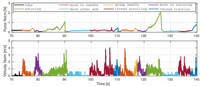
**Fig. 3:** HMM decoding of the robotic surgical re-constructive procedure shown on force norm signal. Different states are shown in different colors.
