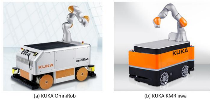
Fig. 1. Industrial mobile manipulator: two representative generations of KUKA mobile manipulator.
