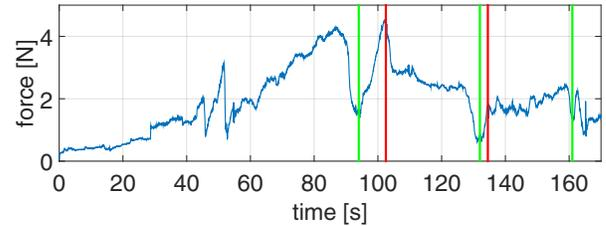
(b) Magnitude of the force due to virtual fixtures. Timestamps marked in green represent the time instances at which the limit switches are pressed, red lines indicate the switch between two virtual fixtures.
