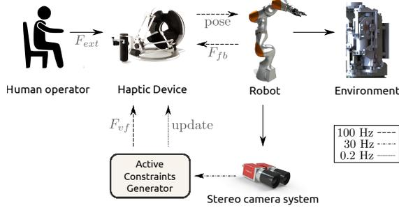
Fig. 4. Block diagram of the overall teleoperation system with virtual fixtures at the master side. The active constraints generator block computes and updates virtual constraints using feature detection algorithms in the images provided by the stereo camera system. Different lines types are intended to show different working frequencies.
