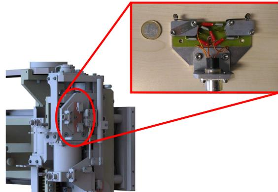
Fig. 1. Two limit switches commonly used in industrial applications: CAD model and related real picture.
