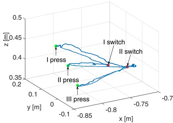
Fig. 6. Robot position (expressed in the robot base frame) recorded during the execution of the considered experimental test with 3 limit switches pressed. Green dots represent the positions of the robot end-effector when limit switches are pressed, while red dots denote the positions in which the switches between two virtual fixtures occur.
