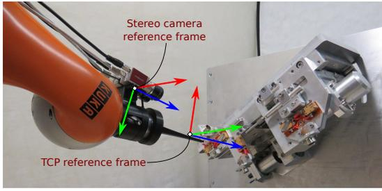
Fig. 2. The slave robot end-effector: the stereo camera and the TCP (Tool Center Point) reference frames.
