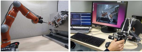
(a) KUKA LWR 4+ and mock- (b) Teleoperator workplace with up of the industrial environment. haptic and visual feedback.
