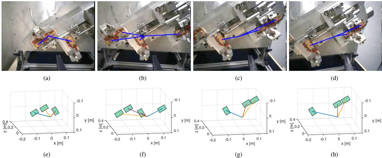
Fig. 8. Key frames taken during the considered experimental test by the stereo camera system located at the slave side (first row) and relative limit switches poses in the stereo camera reference frame (second row). From left to right the operator scans the entire mock-up specifying the robot pose with the haptic device; the virtual fixtures are dynamically computed, consequently updated ((e), (f), (g) and (h)) and shown in the visual feedback to the human operator ((a), (b), (c) and (d)).
