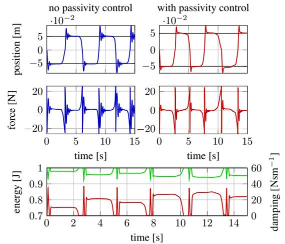
Fig. 3. Comparison between virtual fixture switch procedures with and without passivity control. The graph at the bottom depicts the trends of energy (green) and damping (red) in case of controlled switch.
