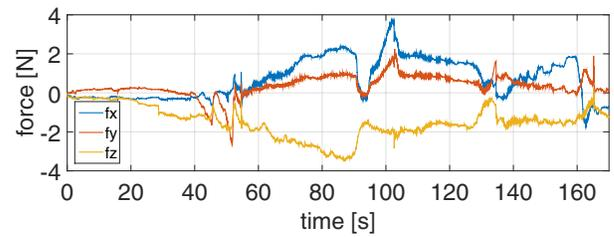
(a) Components of the force rendered by the haptic device due to the virtual fixtures (except for the scale factor  $K_p$ , these components coincide with those of the error between the commanded position and the desired path).
