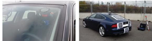
(a) Host vehicle with mounted cameras (left camera) (b) Remote vehicle and DGPS base station
