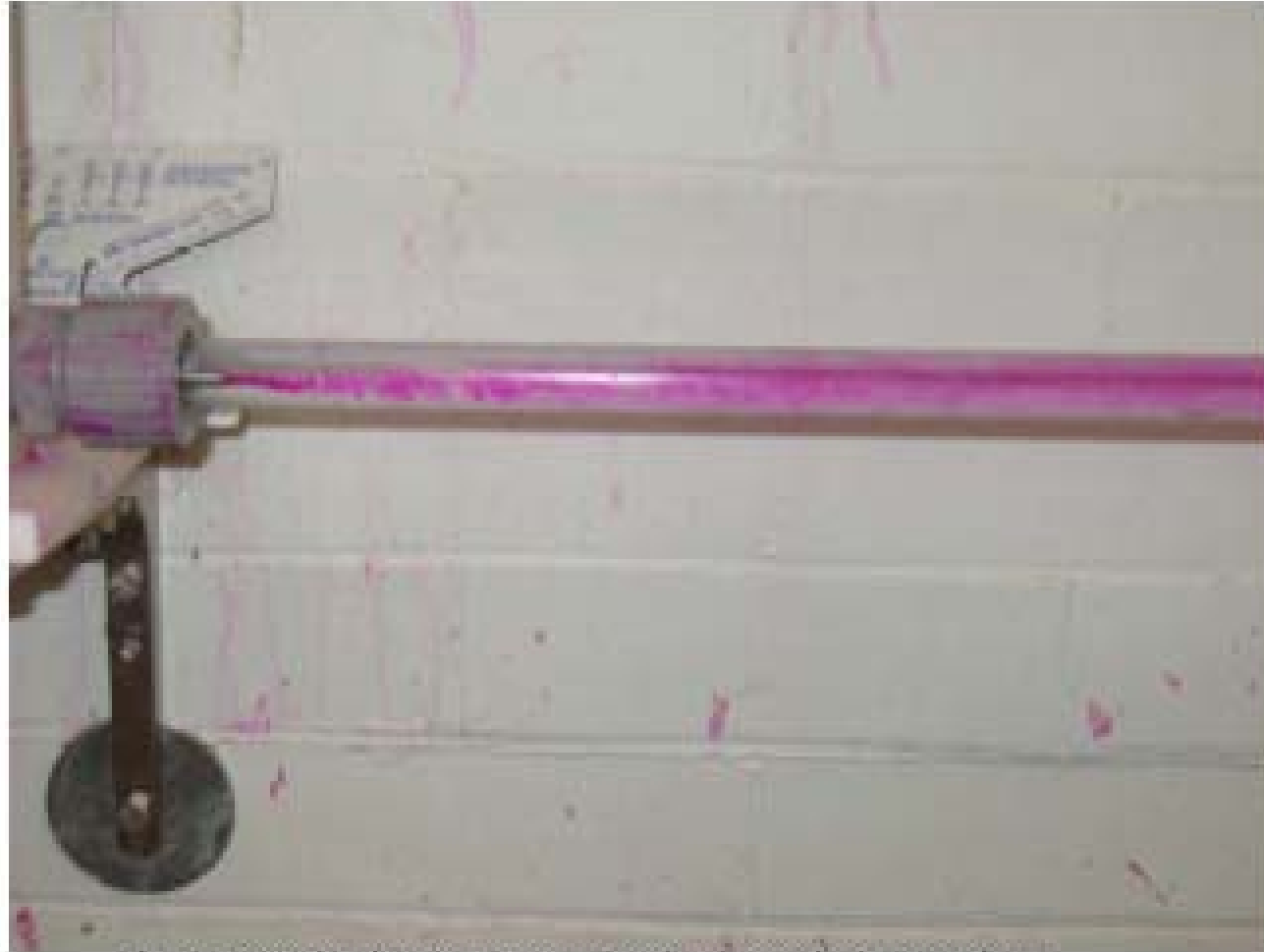
Figure 6: This picture shows flow in the turbulent regime
