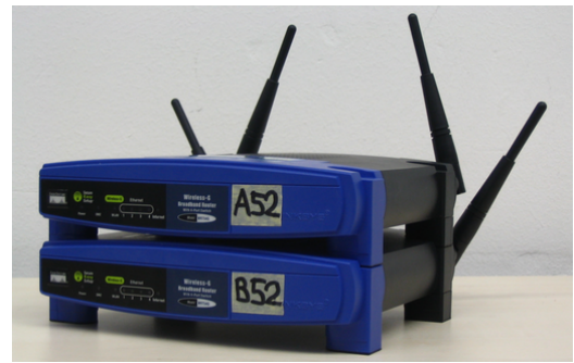
Figure 2: MobiMESH Access Router implementation
