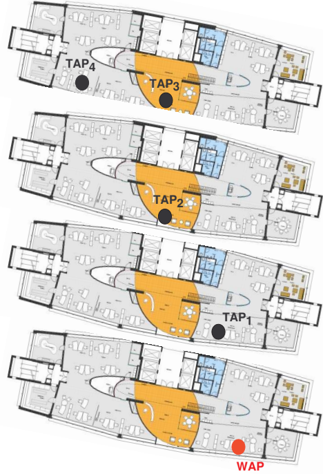
Figure 5: Topology 2: nodes are on adjacent floors.
