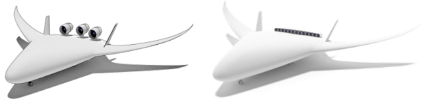
Figure 1. BWB Design Concepts for AGILE EU Project
