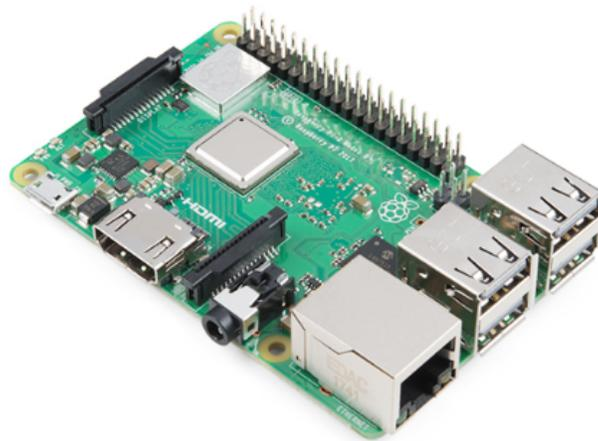
Figura 3.1: Raspberry Pi 3 Model B+
