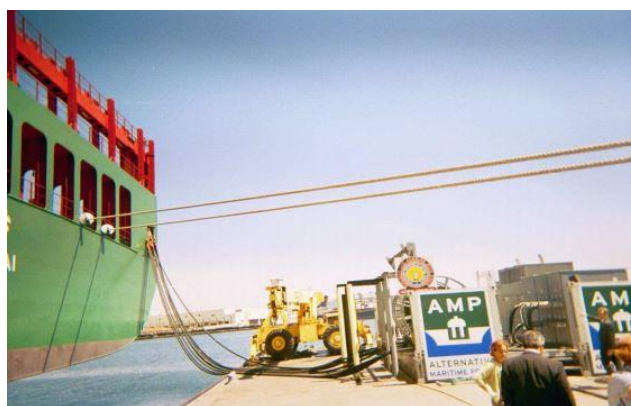
Fig. 4 Cold ironing arrangement in a Chinese port
