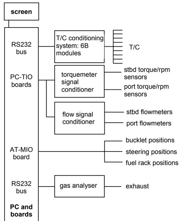
Figure 2 - The data logger
