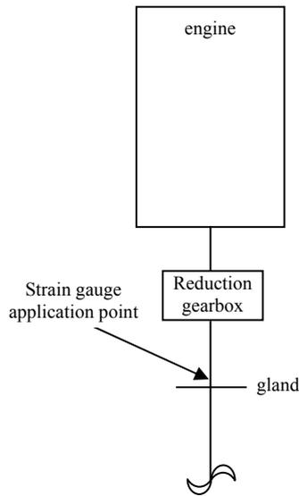
Figure 3 - Position of the torquemeter unit
