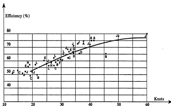
Figure 9 – Typical efficiency results for KaMeWa water-jet propulsion system [7]
