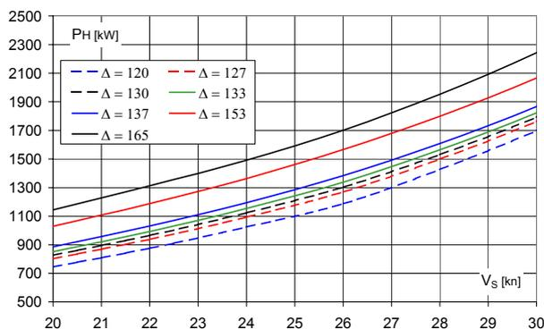
Figure 6 – P<sub>H</sub>: experimental and extrapolated curves
