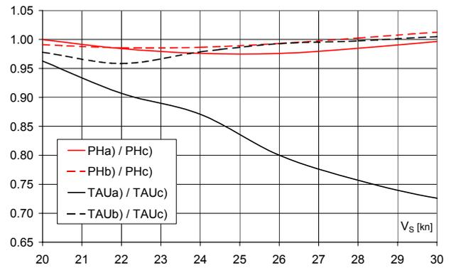
Figure 5 – Effects of the towing position on  $\tau$  and  $P_H$
