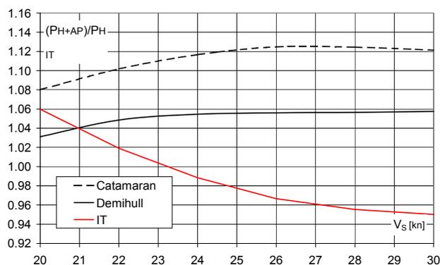
Figure 7 – Influence of the appendages and Total Interference Coefficient
