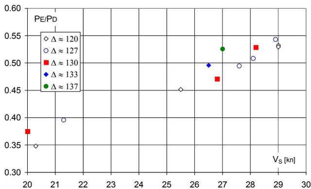
Figure 8 – Synthesis of towing tank and full scale data
