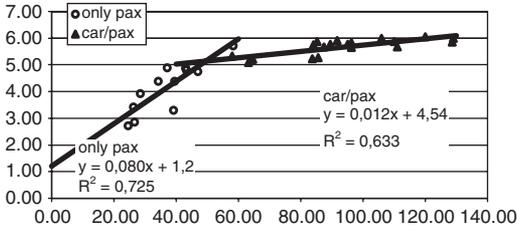
Figure 7.  $L_{WL}/B_{WL}$  vs.  $L_{WL}$  for monohulls.
