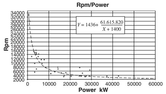
Figure 14. Rpm against power.
