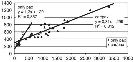
Figure 1. Pass number vs. displacement (t) for monohulls.
