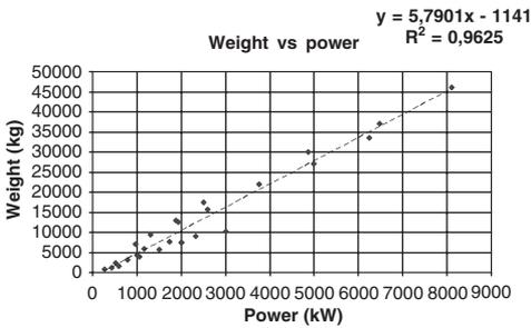
Figure 11. Weight against power L and V dispositions.
