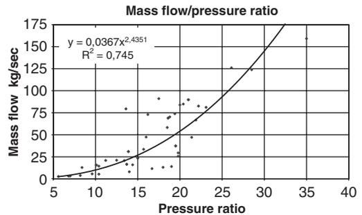
Figure 15. Air mass flow against pressure ratio.
