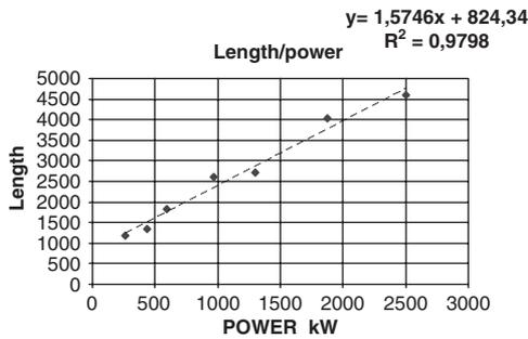
Figure 10. Length (mm) against Power (kw) L disposition.
