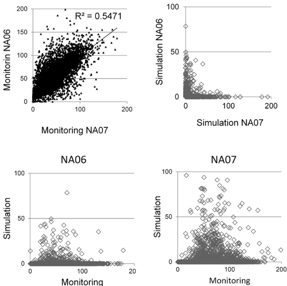
Fig. 11. Correlations between 1-h  $\text{NO}_2$  concentrations. Up correlation between NA6 and NA7: left monitoring data; right simulations. Down correlations between monitoring and simulations: left NA6; right NA7. All values are concentrations in  $\mu\text{g}/\text{m}^3$ .
