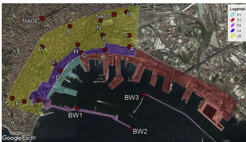
**Fig. 2.** Receptors inside the port and the urban area whose data were compared with simulations: monitoring areas and single receptors.
