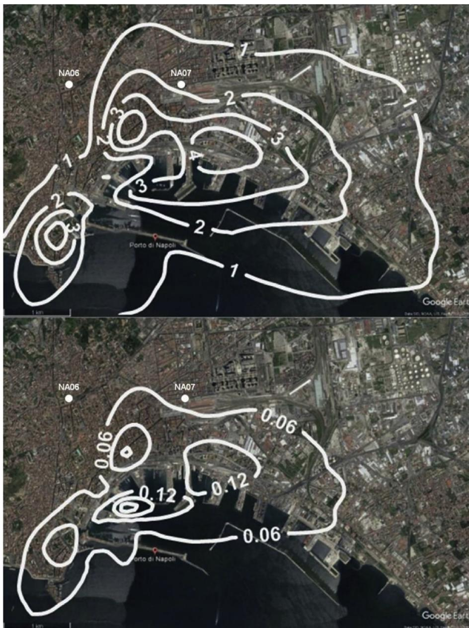
Fig. 8. Simulations: maps of year average [ $\mu\text{g}/\text{m}^3$ ]: up  $\text{NO}_2$ , down  $\text{SO}_2$ .
