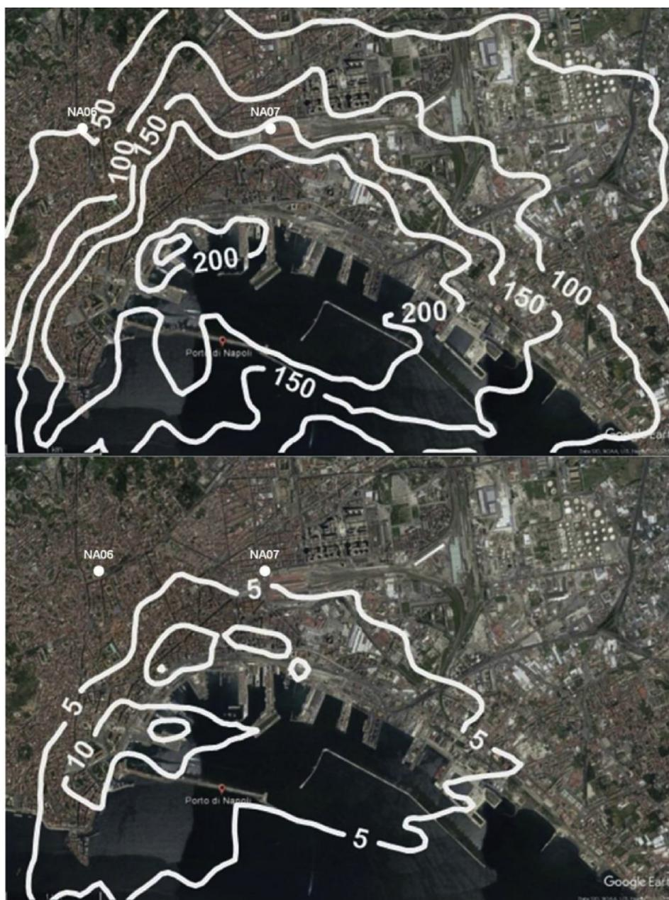
Fig. 9. Simulations: maps of 10th maximum value of 1-h average [ $\mu\text{g}/\text{m}^3$ ]. Up  $\text{NO}_2$ , down  $\text{SO}_2$ .
