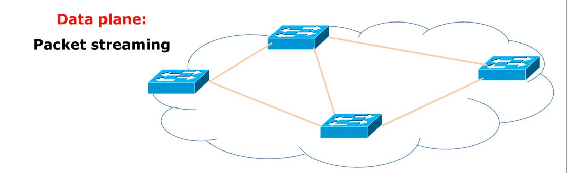
Forward, filter, buffer, mark, rate-limit, and measure packets
