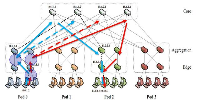
At the first edge switch, traffic from 10.0.1.2 to 10.2.0.3 is randomly routed either on the left path or on the right path Also aggregation switches may randomly choose one among two different paths
