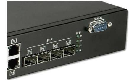
A switch with 4 SFP ports
