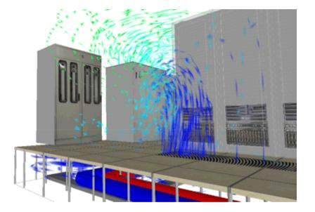
Solution: prevent cold and hot air mix through physical barriers ("containment")
