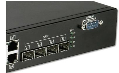
A switch with 4 SFP ports
