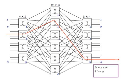
• Example: N=1000, n=10  $\rightarrow$  m=100 switches into the first and third stage
