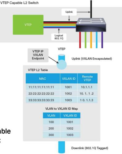
Packets received from a VTEP on the uplink are mapped from the VXLAN ID to an IEEE 802.1Q VLAN ID and sent as Ethernet frames on the downlink to the VM
