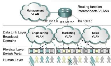
If a hub is connected to VLAN port on a switch, all devices on that hub must belong to the same VLAN
