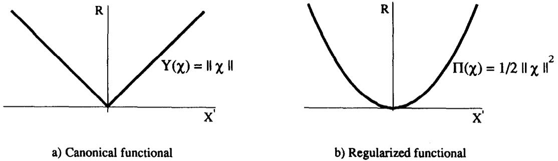
Fig. 7. Yield functionals for von Mises criterion.
