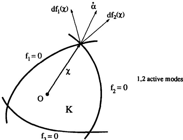
Fig. 5. An inelastic model with three yield modes.
