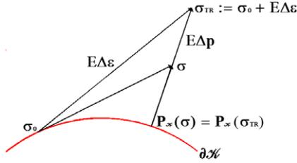
Fig. 2. Geometric scheme of the Duvaut and Lions discrete elastoviscoplastic constitutive law.
