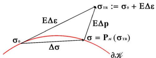
Fig. 1. Geometric scheme of the discrete elastoplastic constitutive law.
