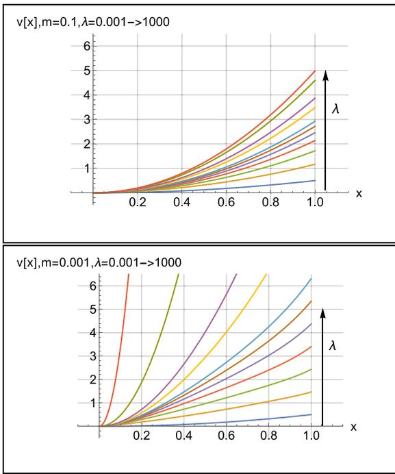
Fig. 5. Mixture strain-driven. Cantilever under uniform bending.  $\lambda = 0.001, 1, 2, 3, 4, 5, 6, 10, 15, 50, 1000$ . Up: elastic deflection for  $m = 0.1$ . Down: elastic deflection for  $m = 0.001$ .
