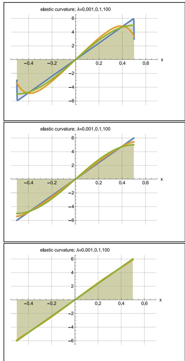
Fig. 7. Stress driven. Clamped beam with transversal end displacement. Top: convolution: no compensation Eq. (7). Middle: boundary effects compensated Eq. (20). Bottom: boundary effects compensated Eq. (27).
