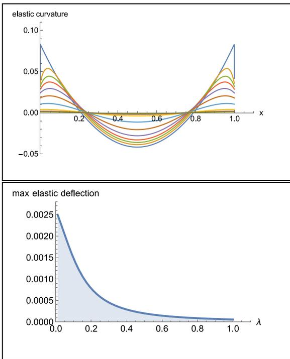
Fig. 6. Stress-driven Eq. (7). Clamped beam under constant loading. Up: elastic curvature for  $\lambda = 0.0001, 0.03, 0.05, 0.07, 0.10, 0.15, 0.25, 0.50, 0.75, 1.00$ . Down: max deflection for  $0 \leq \lambda \leq 1$ .
