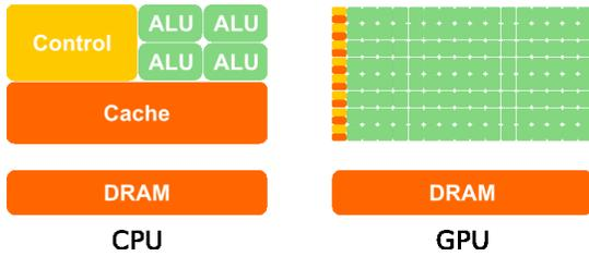
Fig. 1. CPU architecture vs. GPU architecture
