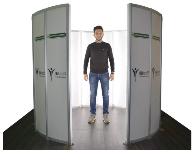
Fig. 1 INBODY, the instant photogrammetric 3D body scanner
