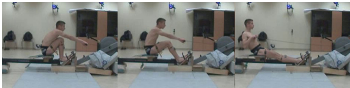
Fig. 7 Three main highlights of a rowing run-test: (left) the catch event; (middle) the instant of minimum load on the sliding seat; (right) the finish event
