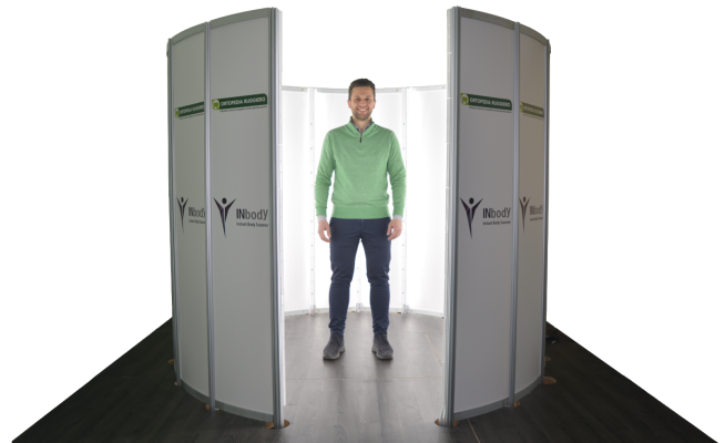
Fig. 1. INBODY, a photogrammetric full body 3D scanner.
