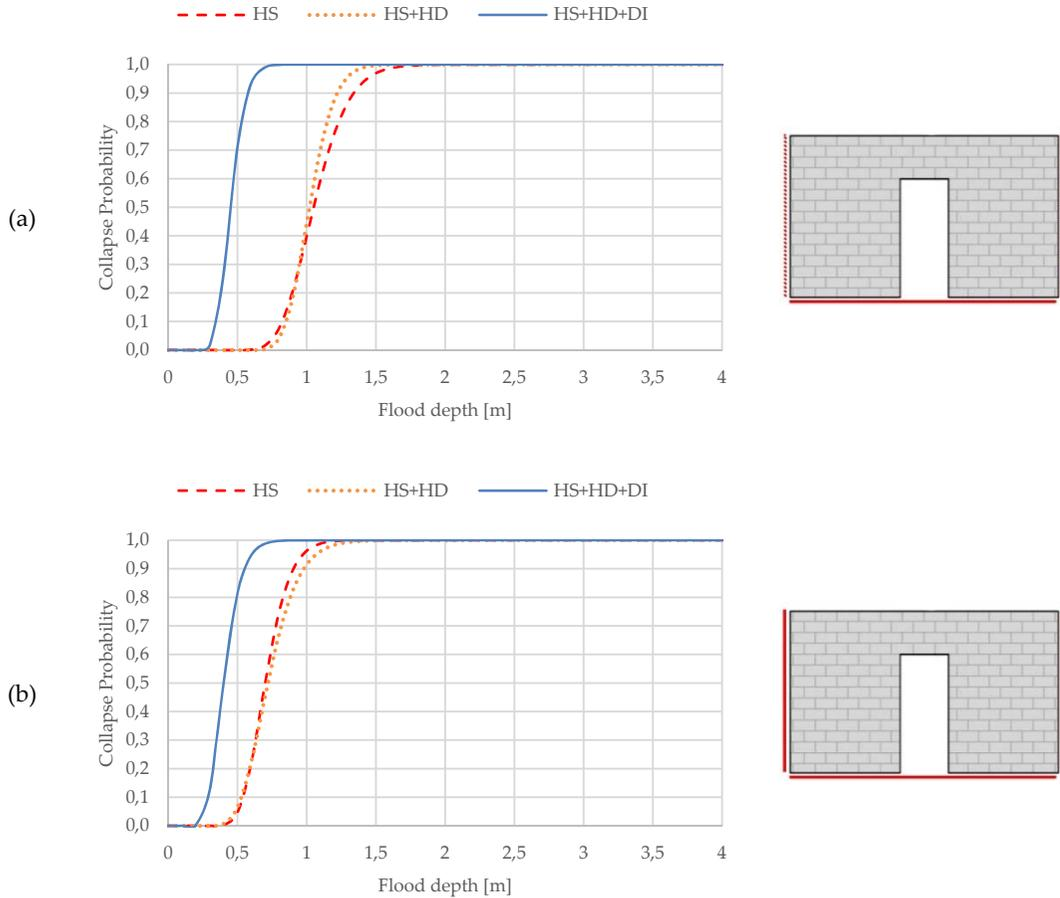
**Figure 4. 18 - Fragility curves for three load combination: (a) hinged-fixed wall with door; (b) fixed wall with door.**
