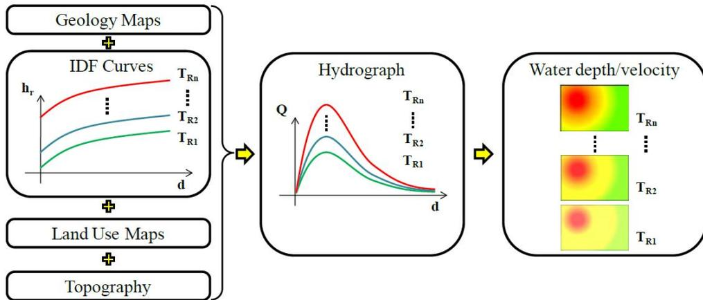
Figure 2. 2: Hydrographic basin modelling procedure.
