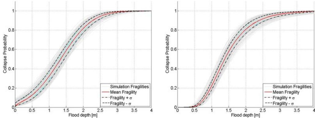
*Figure 4. 13 - Robust fragility curves at CO limit state obtained based on 50 simulations: (left) Normal Cumulative Distribution of probability; (right) LogNormal Cumulative Distribution of probability.*
