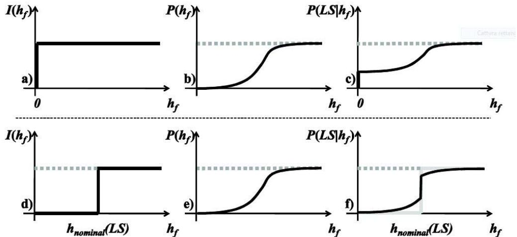
Figure 2. 13 - schematic diagram of: a) step function for SE; b) lognormal CDF for SE; c) three-parameters CDF for SE; d) step function for LS; e) lognormal CDF for LS; f) three-parameters CDF for LS.
