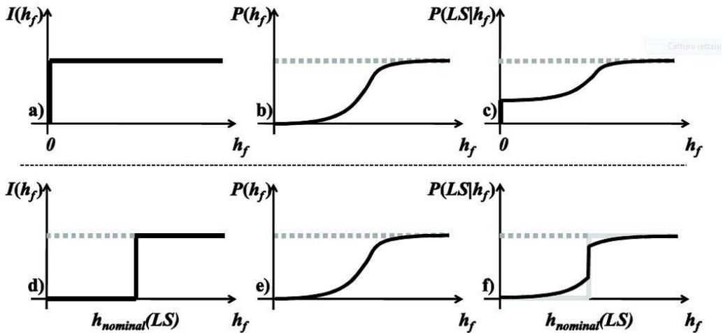
Figure 2. 13 - schematic diagram of: a) step function for SE; b) lognormal CDF for SE; c) three-parameters CDF for SE; d) step function for LS; e) lognormal CDF for LS; f) three-parameters CDF for LS.
