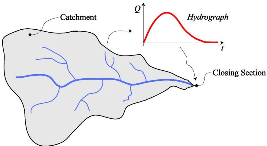
Figure 2. 3: The schematic diagram of a hydrographic basin.
