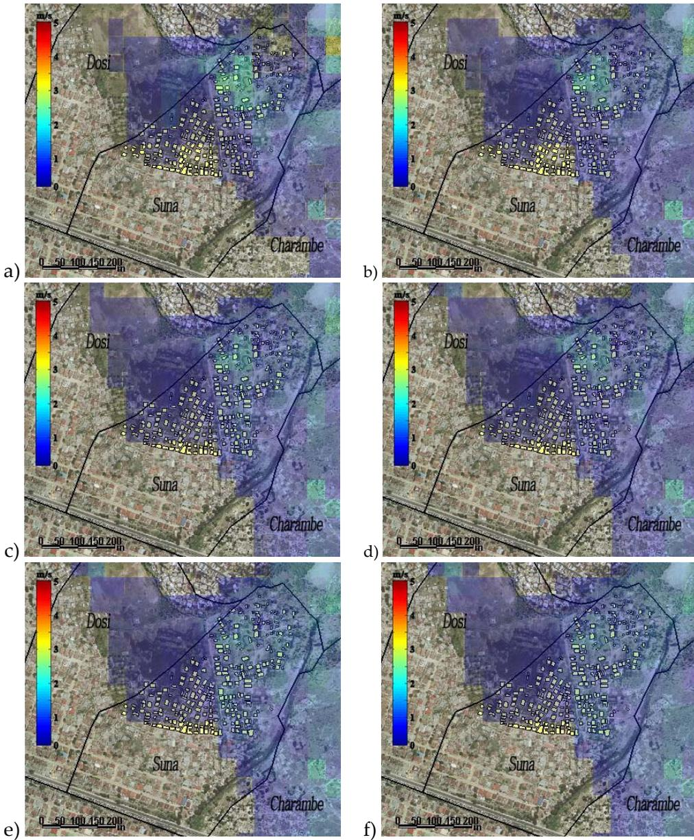
Figure 4.6 – Inundation profiles for different return periods, based on historical data, in terms of  $v_{max}$ : a)  $T_R=2$  years, b)  $T_R=10$  years, c)  $T_R=30$  years, d)  $T_R=50$  years, e)  $T_R=100$  years, f)  $T_R=300$  years.
