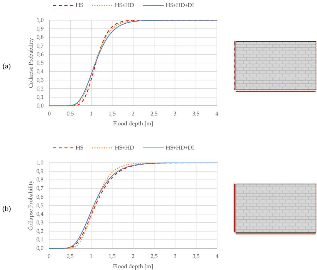
Figure 4. 16 - Fragility curves for three load combination: (a) hinged-fixed solid wall; (b) fixed solid wall.
