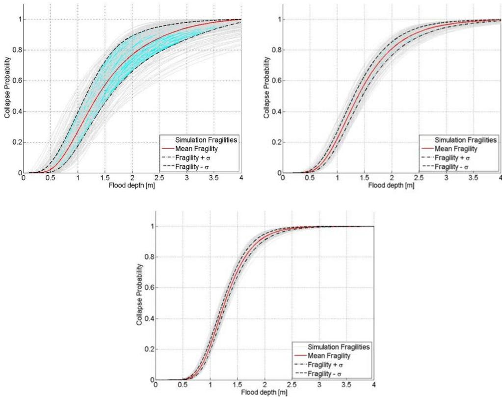
*Figure 4.10 - Robust fragility curves at CO limit state: (I) 10 simulations; (II) 50 simulations; (III) 100 simulations.*
