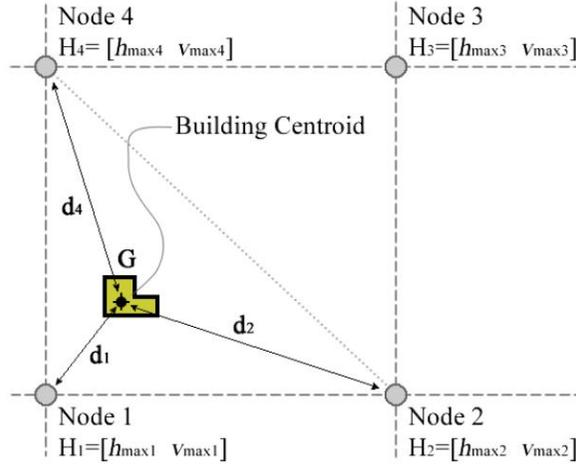
Figure 2. 4: Graphical representation of the spatial interpolation for point G.
