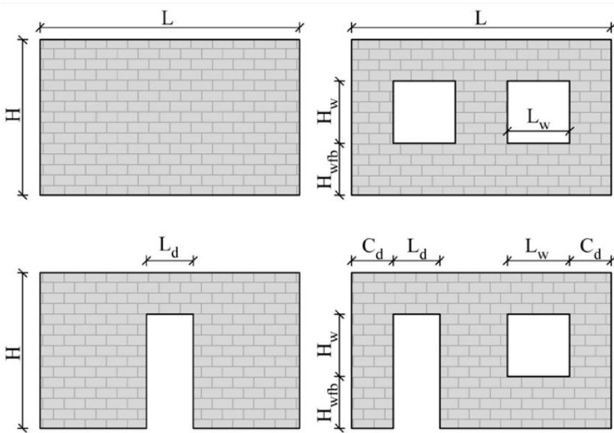
Figure 2. 10: Various models of wall
