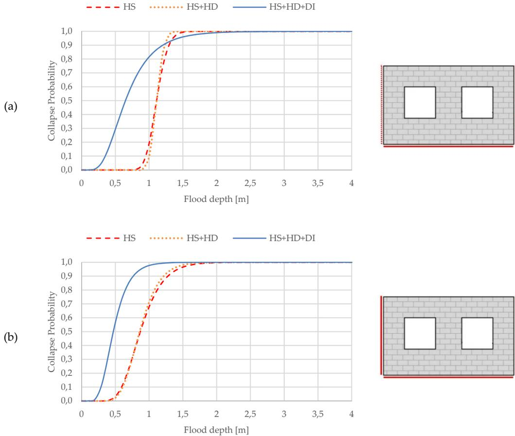
**Figure 4. 17 - Fragility curves for three load combination: (a) hinged-fixed wall with windows; (b) fixed wall with windows.**
