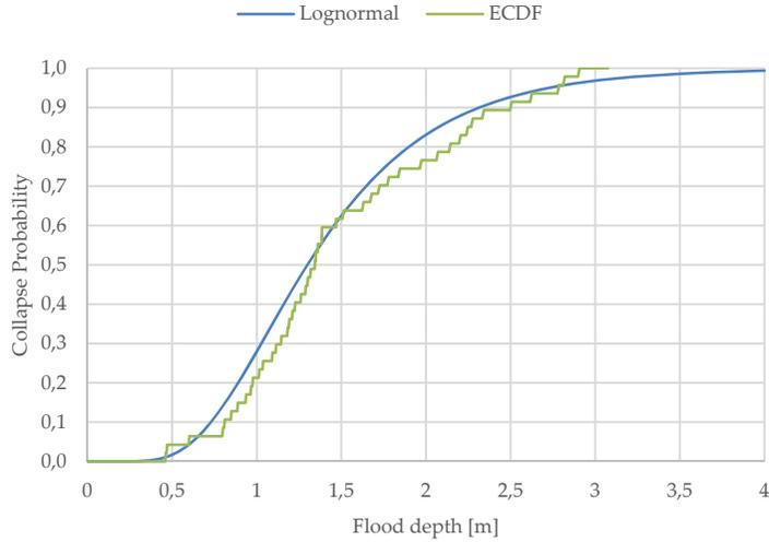
Figure 4.14: Overlaying of Normal, Lognormal and ECDF fragility curves.
