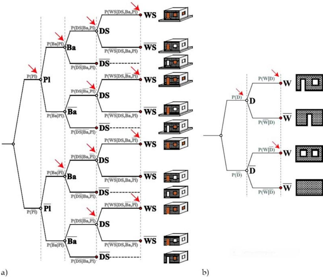
Figure 2. 6: a) logic tree for the waterproofness, b) logic tree for the model generation.
