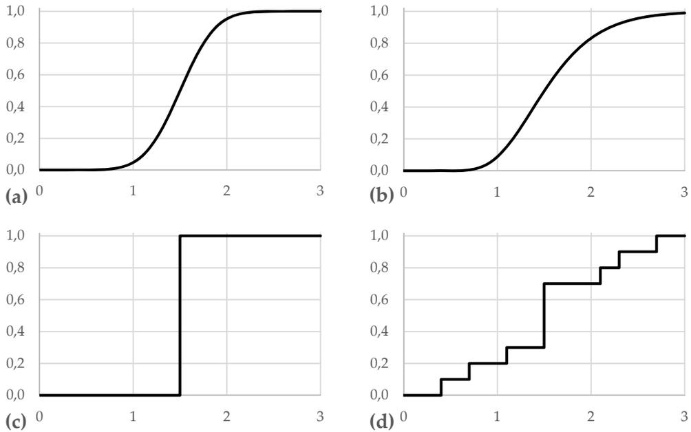
*Figure 3. 8 - Custom fragility curves: a) normal CDF; b) lognormal CDF; c) nominal step function; d) totally custom fragility curve.*
