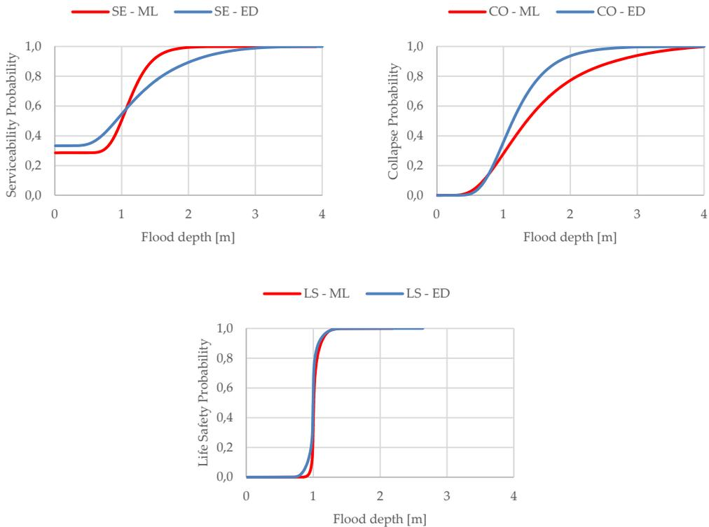
**Figure 4. 11 – Overlay of the median fragility for the three limit state considered for two typology of extraction with 10 analysis simulations.**
