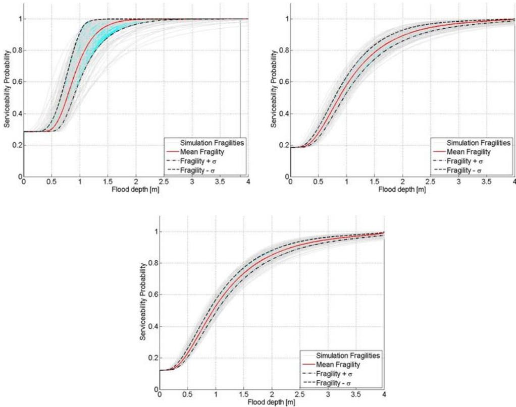
**Figure 4. 9 - Robust fragility curves at SE limit state: (I) 10 simulations; (II) 50 simulations; (III) 100 simulations.**
