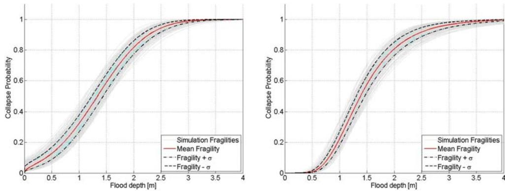
**Figure 4. 13 - Robust fragility curves at CO limit state obtained based on 50 simulations: (left) Normal Cumulative Distribution of probability; (right) LogNormal Cumulative Distribution of probability.**
