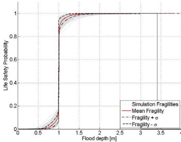
Figure 4. 21: Robust fragility curve at Life Safety limit state.
