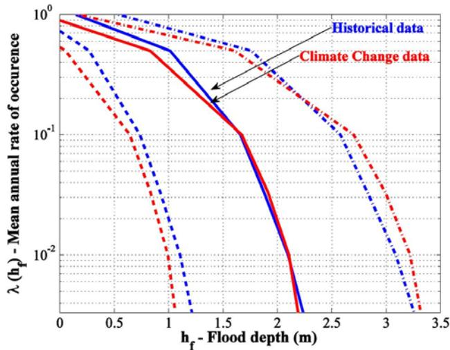
Figure 4. 4: Overlaying representative (mean and mean +/- standard deviation) hazard curves obtained based on, historical data (blue curves) and climate projections (red curves).
