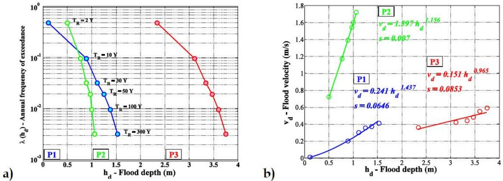
Figure 2. 5: a) Hazard curves; b) Flood height versus flood velocity power-law relation.
