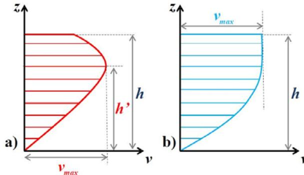
Figure 2. 8: a) real velocity profile; b) approximate velocity profile.
