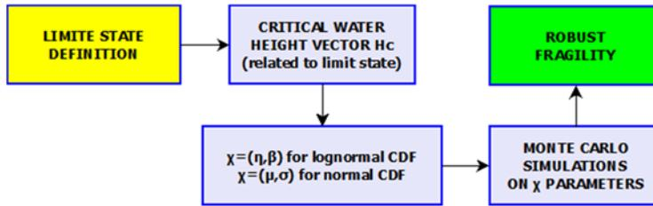
Figure 3. 6: VISK fragility evaluation procedure.
