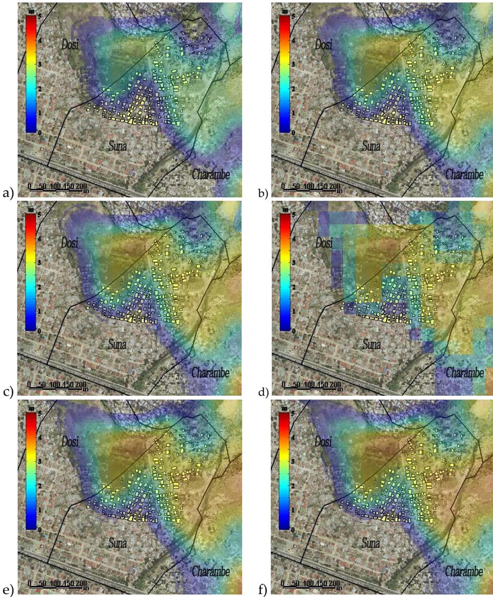
Figure 4.5 – Inundation profiles for different return periods, based on historical data, in terms of  $h_{max}$ : a)  $T_R=2$  years, b)  $T_R=10$  years, c)  $T_R=30$  years, d)  $T_R=50$  years, e)  $T_R=100$  years, f)  $T_R=300$  years.
