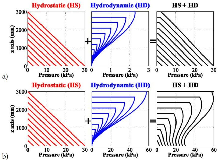
Figure 2. 9: Hydrostatic and hydrodynamic pressure profile for two different pairs of parameters: (a) low flooding height and low velocity; (b) low flooding height and high velocity.
