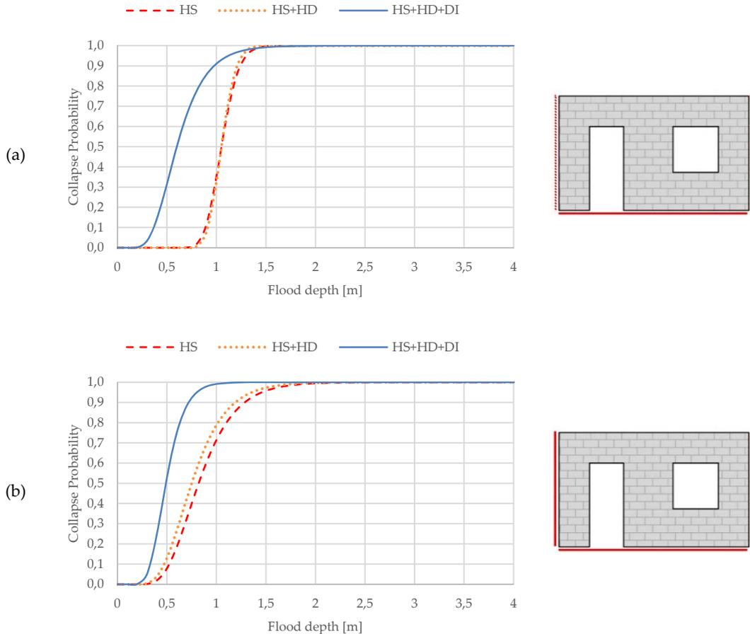
**Figure 4.19 - Fragility curves for three load combination: (a) hinged-fixed wall with door and windows; (b) fixed wall with door and windows.**
