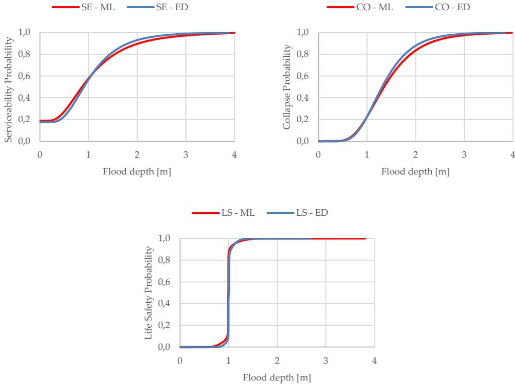
**Figure 4.12 – Overlay of the median fragility for the three limit state considered for two typology of extraction with 50 analysis simulations.**
