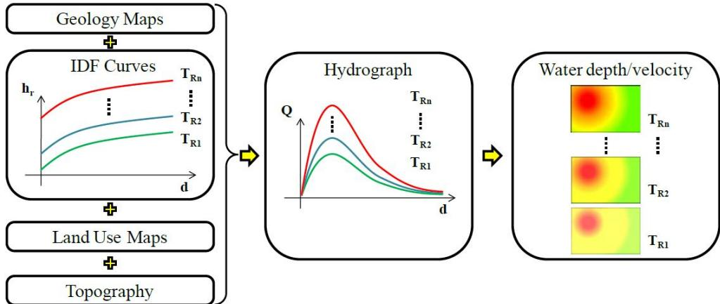
*Figure 2.2: Hydrographic basin modelling procedure.*
