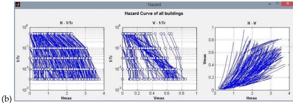
Figure 3. 2 – (a): hazard data on the map viewed as surf; (b): hazard curves.
