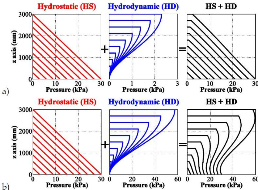
*Figure 2. 9: Hydrostatic and hydrodynamic pressure profile for two different pairs of parameters:
