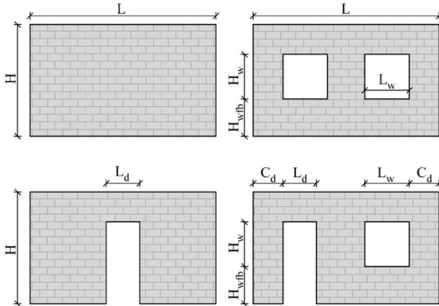
*Figure 2. 10: Various models of wall*
