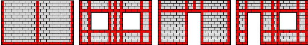
Figure 2.11: Zones of panel in which is searched the critical section.
