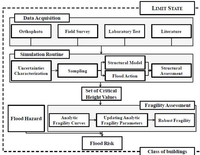
*Figure 2.7: Procedure used to vulnerability assessment.*
