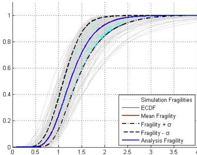
*Figure 3. 7: Example of VISK robust fragility curve.*
