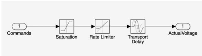
Fig. 4. CC power supply model used for performance assessment.
