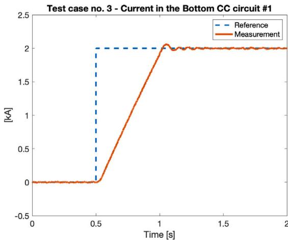
Fig. 7. Current in Bottom CC circuit for Test case no. 3.
