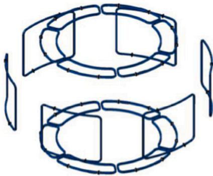
Fig. 1. The 18 ITER superconductive Correction Coils (CC). The coils are placed at three different vertical positions.
