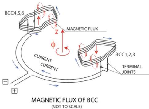
Fig. 2. Schematic of the connection of two bottom CC.
