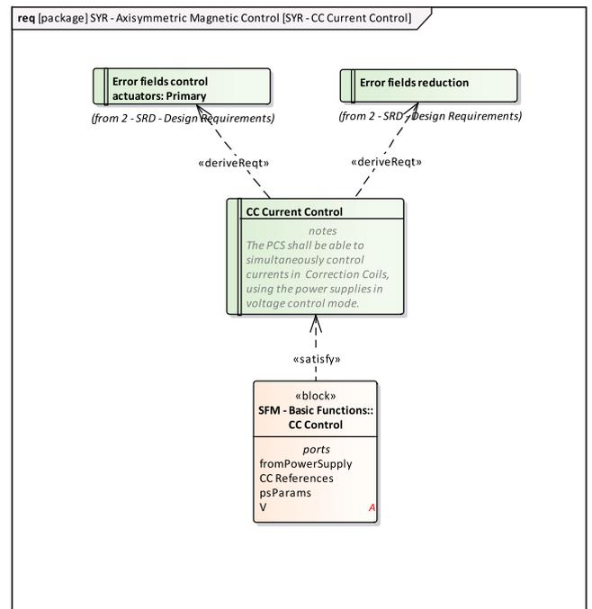
Fig. 3. SYR requirements for the CC Control block and its relation with SRD requirements.
