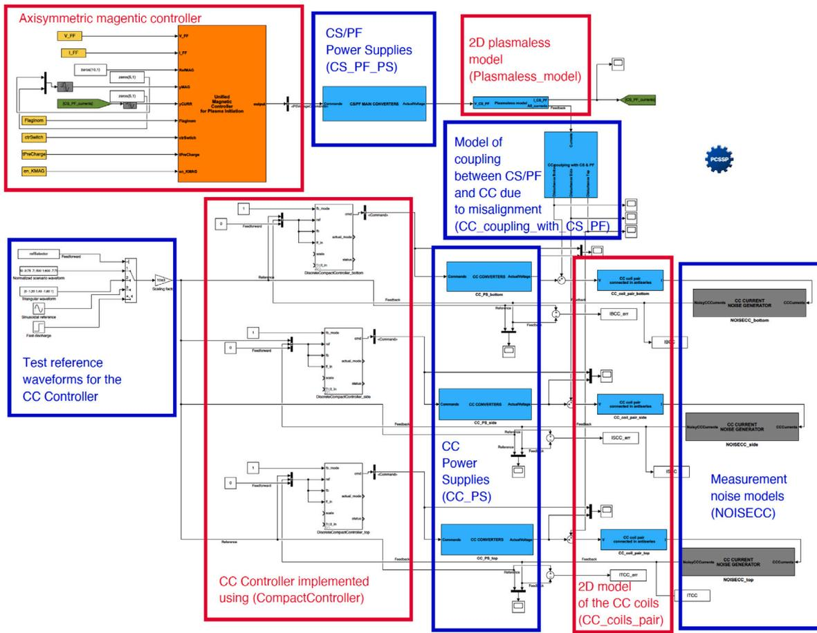
Fig. 6. Simulink PCSSP-compliant model used to run the simulations that correspond to the Test cases no. 1 and no. 2 reported in Table 3.
