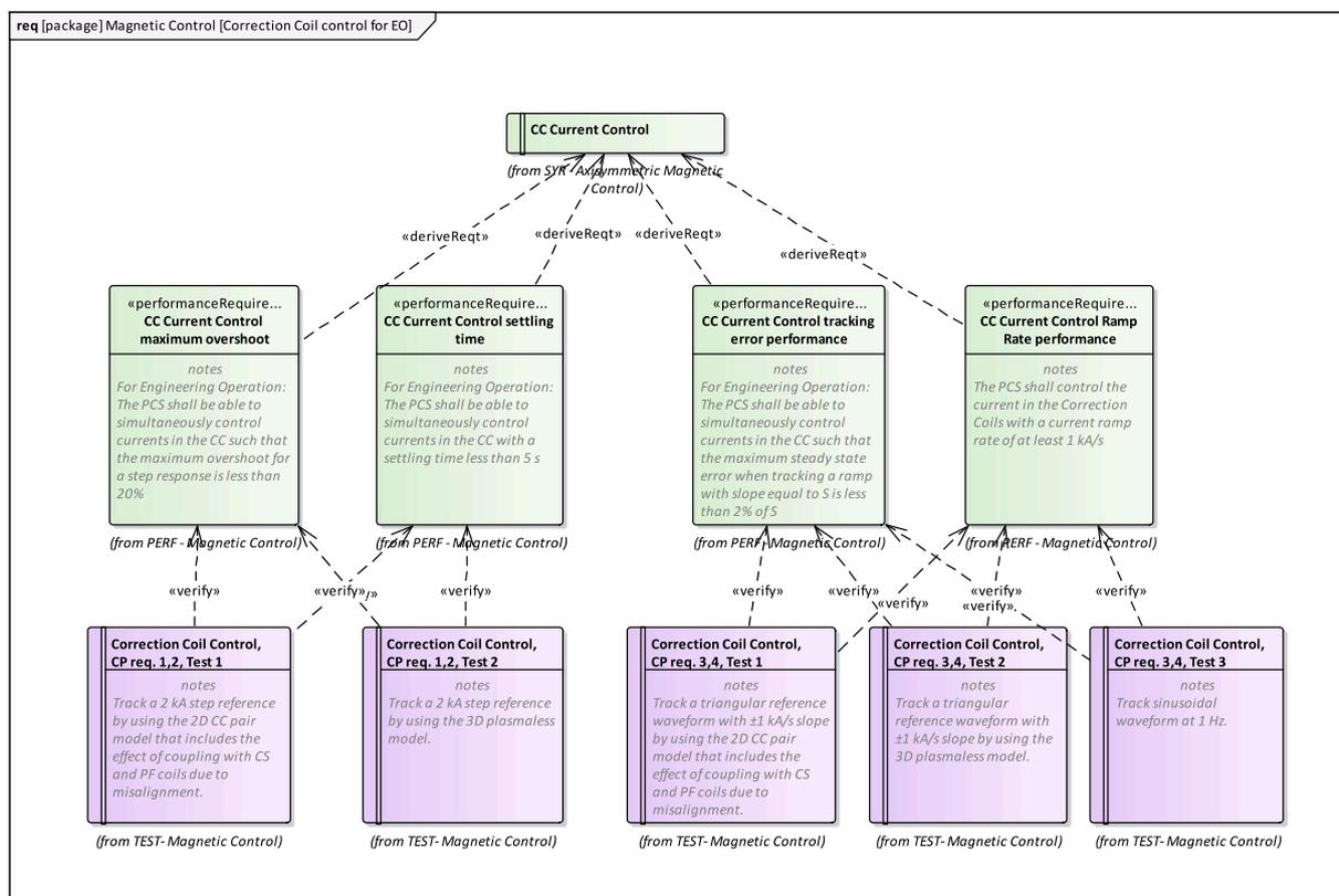
Fig. 5. Test cases and their relationships with Performance Requirements listed in Table 1.
