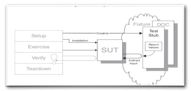
**Q:** How can we verify logic independently when it depends on indirect inputs from other software components?
