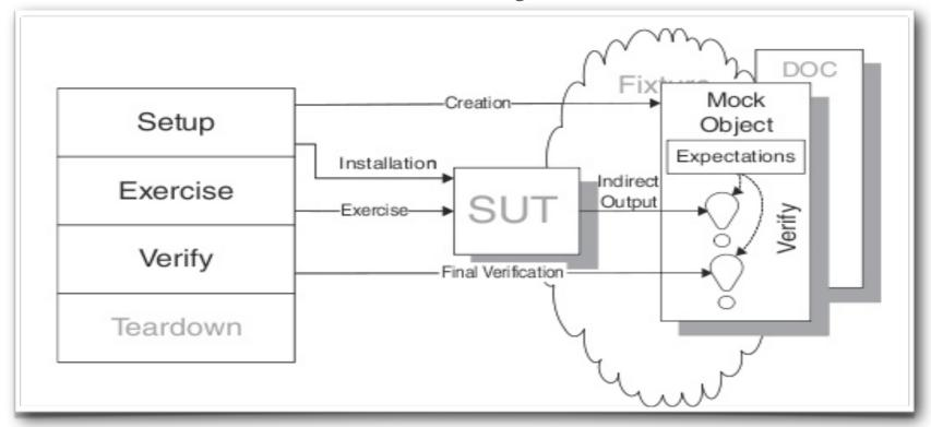
**Q:** How can we implement Behavior Verification for indirect outputs of the SUT?
