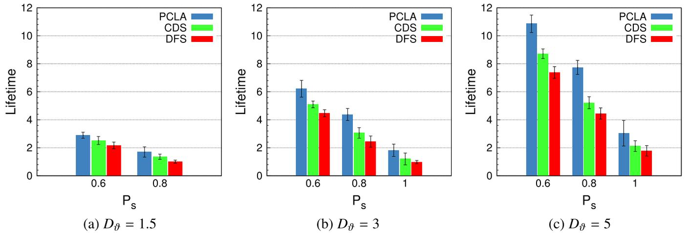
Fig. 12. Impact of coverage requirement ( $P_s$ ) on the network lifetime for different values of  $D_\theta$ . Increasing coverage requirements has a negative impact on the lifetime of all the algorithms.
