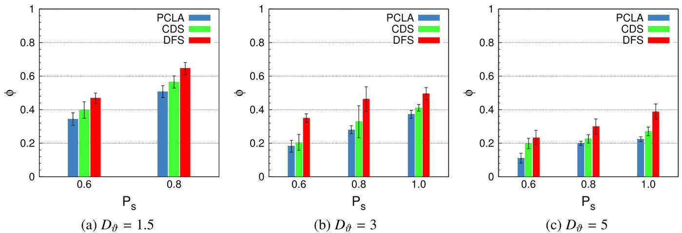
**Fig. 7.** Impact of coverage requirement ( $P_s$ ) on Working-Node Ratio ( $\phi$ ) for different values of  $D_\theta$ . Increasing coverage requirements has a detrimental impact on the performance of all the algorithms, with  $\phi$  exposing an increasing trend on average for increasing values of  $P_s$ . This impact is mitigated by deploying a larger number of nodes, i.e. for greater values of  $D_\theta$ .
