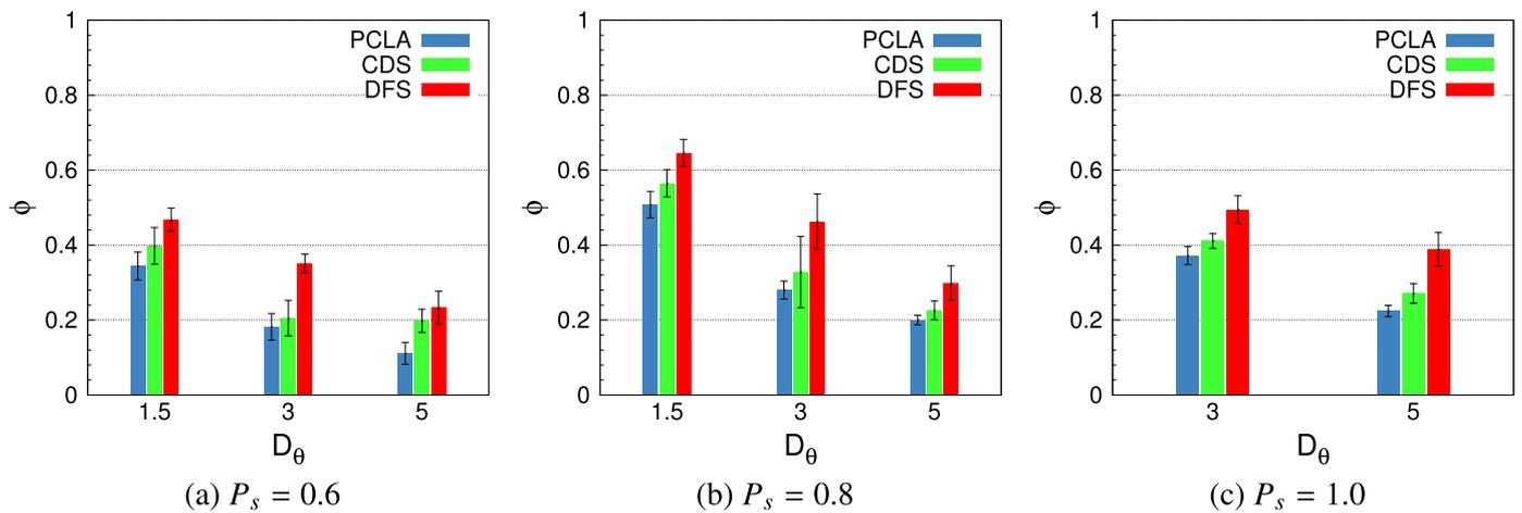
**Fig. 6.** Impact of average region coverage degree ( $D_\theta$ ) on working-node ratio ( $\phi$ ) for different values of  $P_s$ .  $\phi$  exposes a decreasing trend on average for increasing values of  $D_\theta$ . PCLA outperforms the other two algorithms in all the circumstances taken into account.
