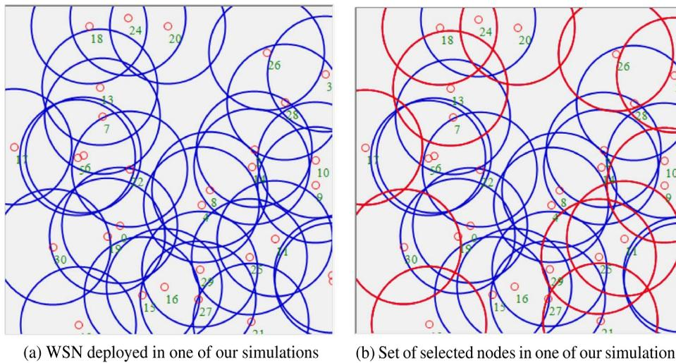
**Fig. 5.** Results of an example simulation. The circles around the nodes indicate their sensing range, while the numbers their IDs. Nodes selected by PCLA are depicted with red circles. (For interpretation of the references to color in this figure legend, the reader is referred to the web version of this article.)
