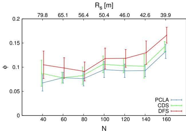
**Fig. 10.** Effect of varying the number  $N$  of nodes, keeping  $D_b$  fixed ( $D_b = 5$ ,  $P_s=0.6$ ). Increasing the number of nodes—and reducing the sensing ranges accordingly—leads to worse results in terms of  $\phi$ .
