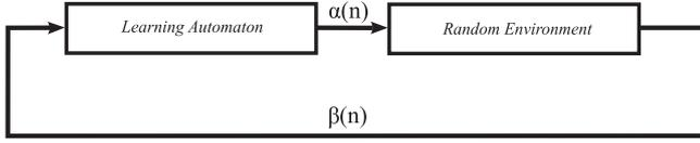
**Fig. 2.** The relationship between the learning automaton and the random environment. The automaton learns to optimally choose actions  $\alpha(n)$  based on the reinforcement signals  $\beta(n)$  provided by the environment.
