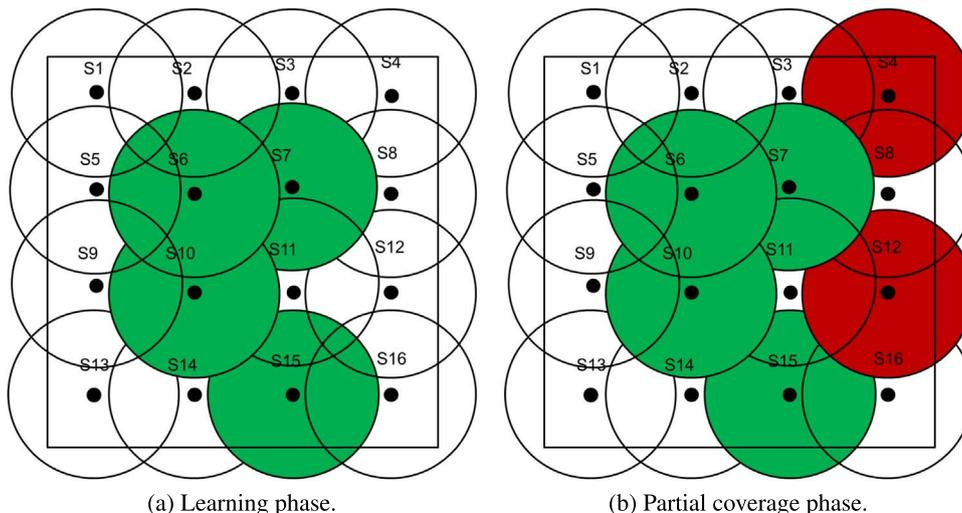
**Fig. 3.** An illustrative example of the selection of nodes in PCLA. The two main phases of our algorithm are highlighted. Nodes selected in the learning phase are colored in green, whereas those selected in the partial coverage phase in red. (For interpretation of the references to color in this figure legend, the reader is referred to the web version of this article.)
