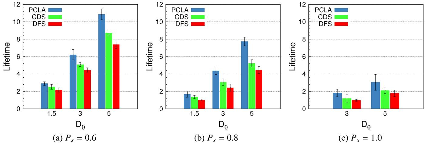
Fig. 11. Impact of average region coverage degree ( $D_\theta$ ) on network lifetime for different values of  $P_s$ . The adoption of PCLA prolongs the network lifetime in all the circumstances taken into account.
