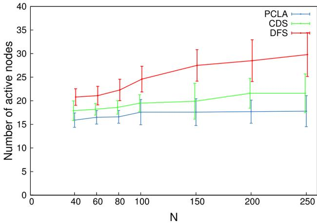
**Fig. 9.** Number of active nodes for different network sizes ( $P_s=0.8$ ,  $R_s = 50$  m). When more nodes are available, all the algorithms settle to slightly worse solutions in terms of number of active nodes.
