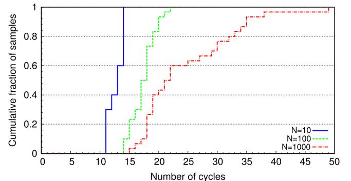
**Fig. 4.** Distribution of the number of cycles ( $I$ ) required by PCLA for WSNs having different number of nodes ( $N$ ). The number of cycles needed by the algorithm is markedly lower than the number of nodes for WSNs having a realistic number of nodes ( $N = 100, 1000$ ).
