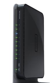
**Netgear WNDR3700** 680Mhz MIPS CPU 64 MB RAM 8MB Flash
