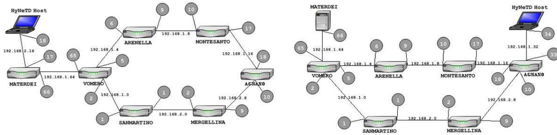
Fig. 5. Ring (left) and Backup (right) topology
