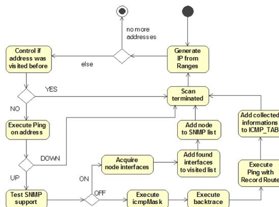
Fig. 3. Scanning thread activity diagram.
