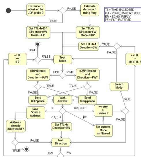
Fig. 4. Backtrace activity diagram.
