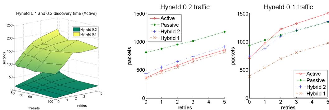
Fig. 6. Ring topology: Discovery time in Active condition (left), Traffic generated by discovery process (right)
